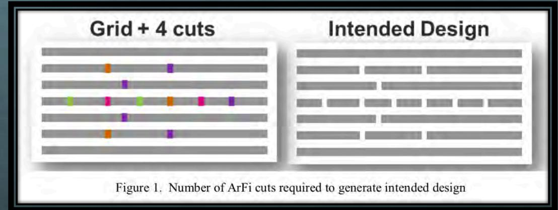
Figure 1. Number of ArFi cuts required to generate intended design
