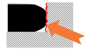
Conclusion: Small difference in diameter combined with the sharp kink on the edge profile contributed to the high defectivity.
