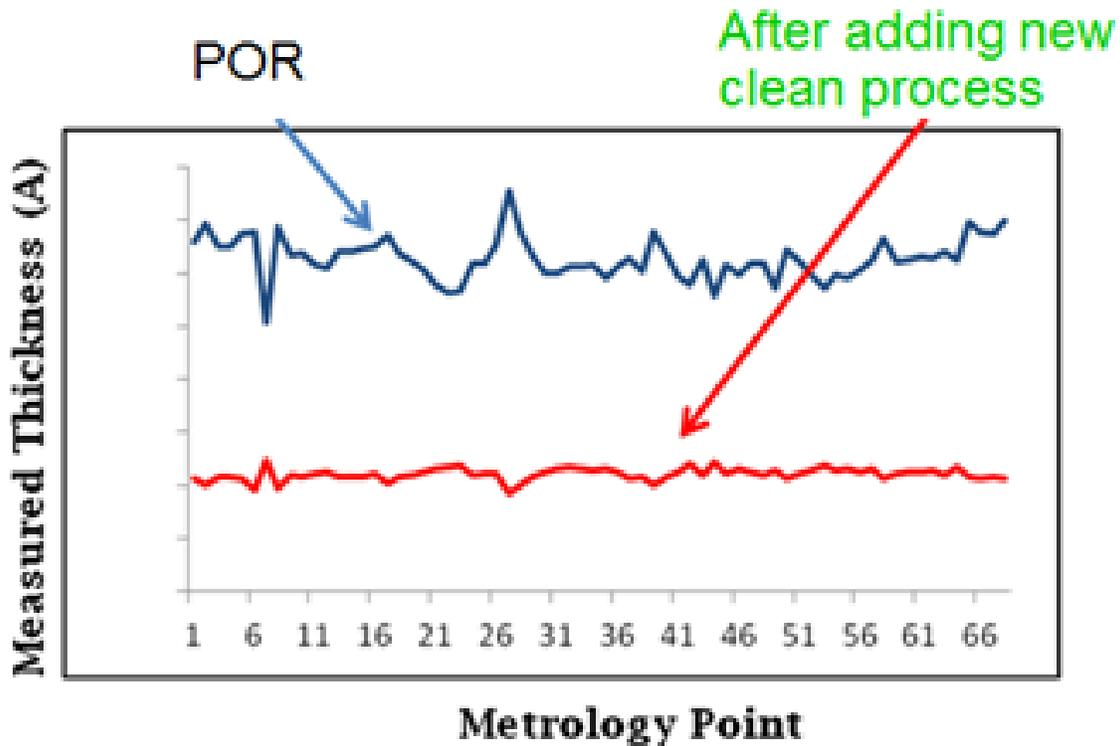
There is one challenge since GCIB is a micro-etching process, there is some surface roughing after the GCIB process. This is being addressed and removed in the next downstream step, poly open wet clean. A very interesting technique that is sure to bring value to the process. They did not disclose anything new about the wet clean, so it was believed that the standard suite of chemistries were being utilized.
